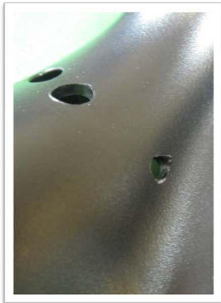
Holes with excess plastic
