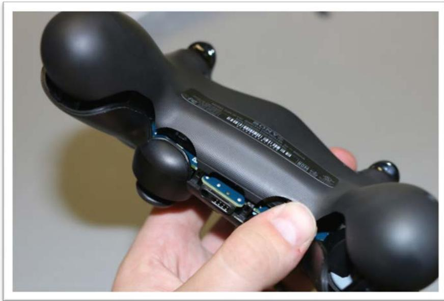
Once the rear handles have cleared the pegs, it is possible to push the back half of the shell “forward” to clear the bumper and triggers, without causing the triggers to pop off. Practice will make this process go more smoothly. If the triggers pop off, **LOOK AROUND CAREFULLY FOR THE SMALL TRIGGER SPRING.** The small trigger spring is required otherwise the trigger will not return fully to the non-pressed position.
