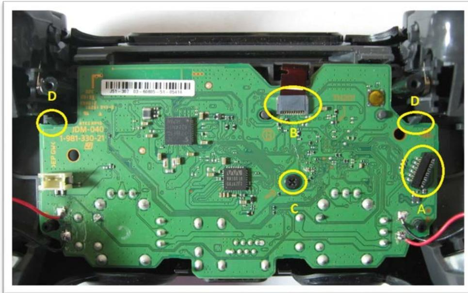
You now need to separate the circuit board from its frame underneath:
