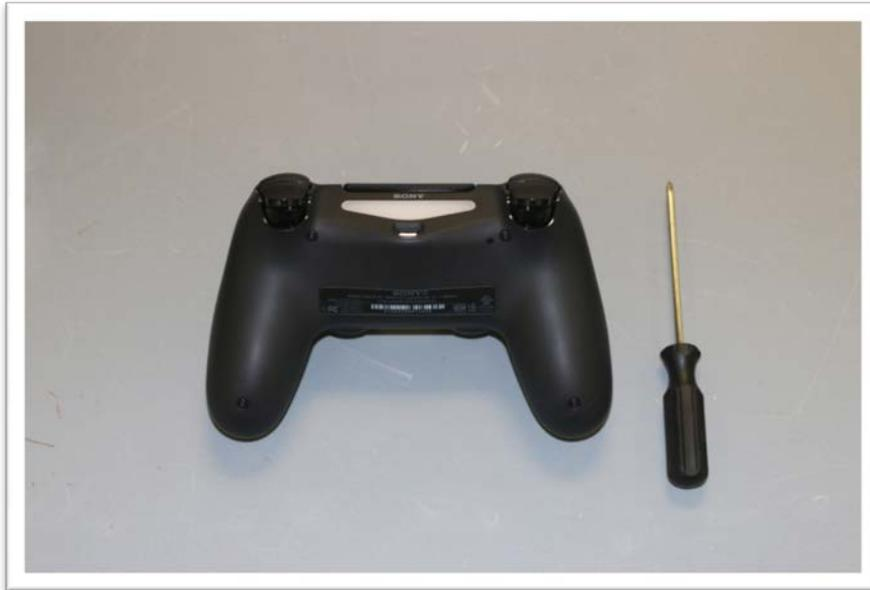
Once the 4 screws are removed, start separating the cover near the microphone port at the bottom. It may take some force to separate the shell. Cracking noise may be heard and some small tabs may be broken in the process, practice will make this process go more smoothly:
