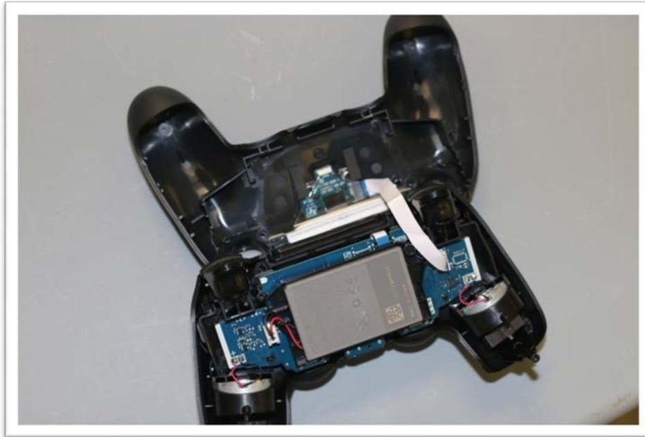
Unhook the battery wires from the battery wires hook and remove the battery by pulling up on white battery connector on the circuit board.
